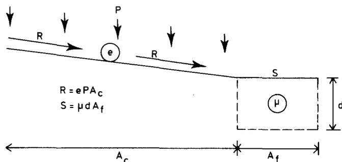
Fig. 2. Diagram showing factors determining surface runoff from catchment area and storage of harvested water.  $A_c$ , size of contributing area (m<sup>2</sup>);  $A_f$ , size of collecting area (m<sup>2</sup>);  $P$ , depth of rainfall (m);  $d$ , depth of storage (m);  $e$ , runoff efficiency;  $\mu$ , storage coefficient;  $R$ , volume of runoff (m<sup>3</sup>);  $S$ , volume of storage (m<sup>3</sup>).
