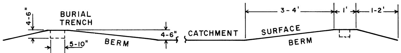
Fig. 3. Berm shape for sides of catchment area.
