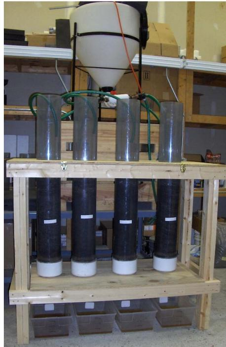
Figure 1: Photo of Column Setup
