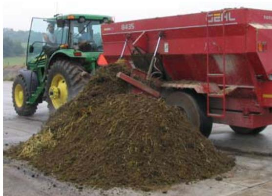
**Figure 4.** The actual windrow can be built using a front end loader or mixing wagon
