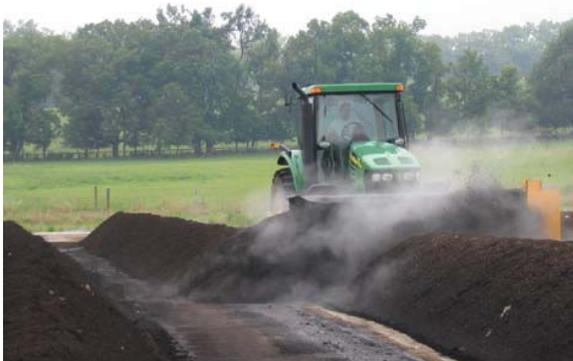
Figure 6. Turning compost with a mechanical turner.
