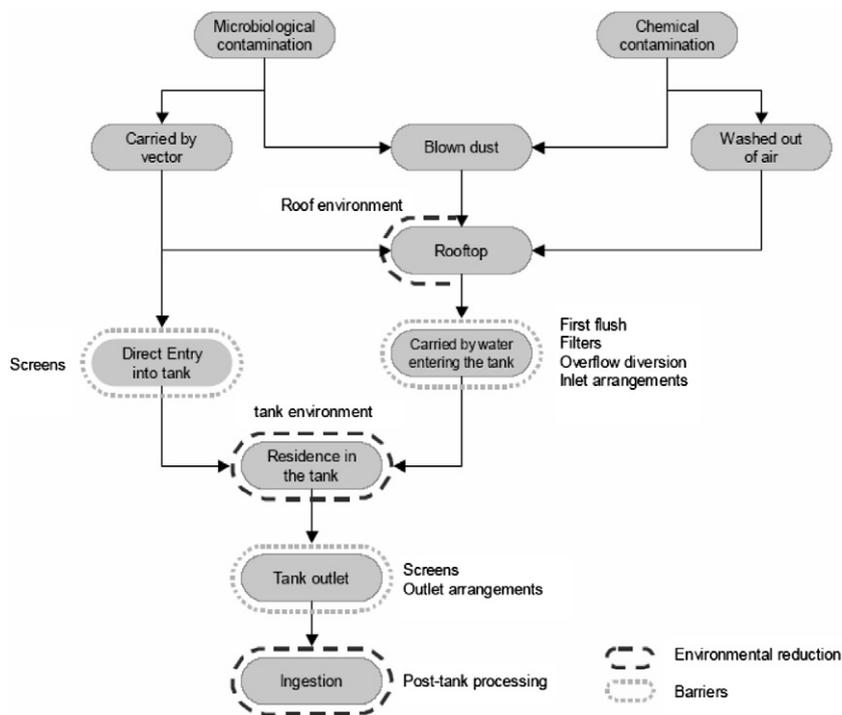
Fig. 2. Contamination paths DRWH systems collecting water from rooftop.
