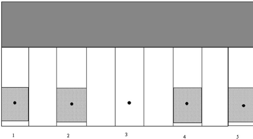
Figure 1. Drawing of shade study layout. Position 3 was location of weather station that monitored wind speed, relative humidity, solar radiation, and ambient temperature as reference for treatments. The treatment locations were 1) 100%, 2) 60%-silver, 3) open (no-shade), 4) 60%-black, 5) snow fence. The grey region at the top of the figure represents an existing metal livestock housing building.
