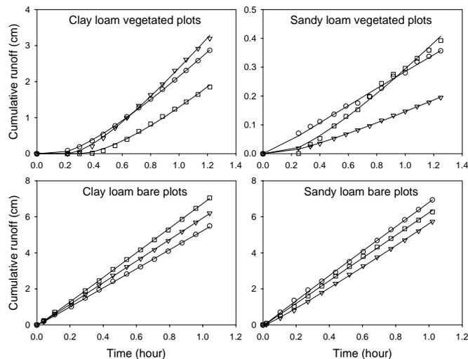
Figure 1. Results of the runoff and infiltration module calibration. Different symbols show replications in measurements, lines show simulation results.
