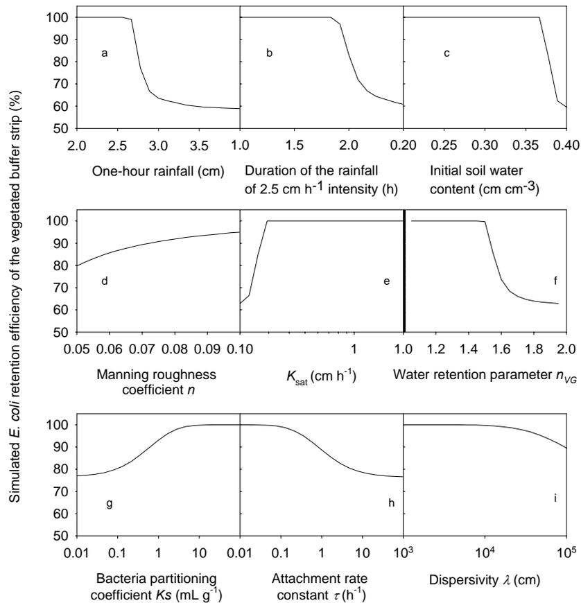
Figure 3. Sensitivity of the vegetated filter strip efficiency to model parameters and rainfall characteristics.
