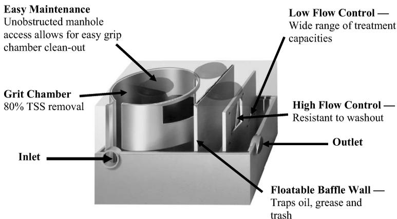
**Figure 1:** Vortechs stormwater treatment system (Stormwater 360, formerly Vortechtechnics, Inc.).
