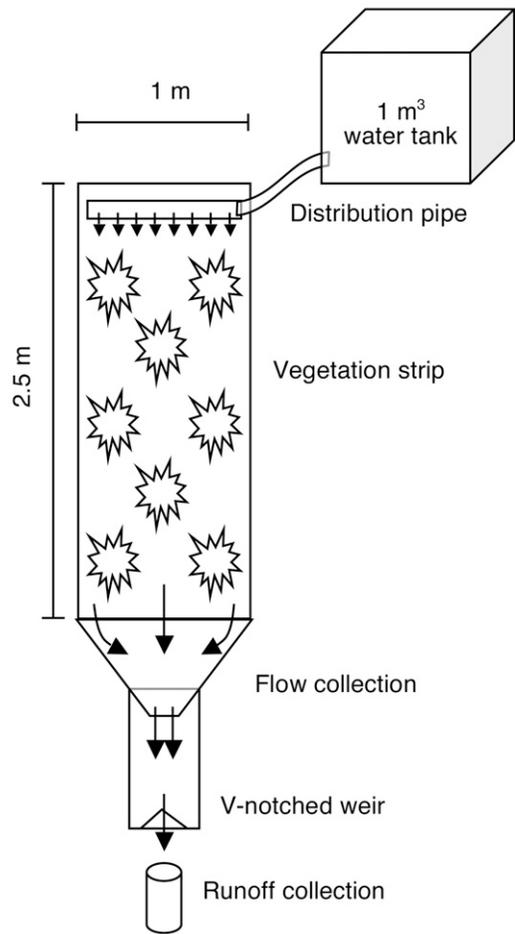
Fig. 1. Schematic of field-based experimental setup showing the plot arrangement, water supply, and runoff collection.
