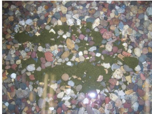
Figure 2. Dispersed manure particles remaining on the bottom of the flume after the cessation of sampling.
