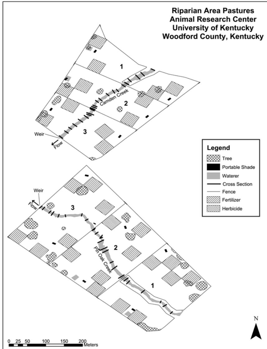
Figure 1. Base Map of Pasture Plots. Plot 1 treatment is the BMPs and a fenced riparian area to exclude cattle from the stream except at a 3.7 m crossing; plot 2 treatment is BMPs with free stream access; and plots 3 are free stream access with no BMPs (control) except for herbicide, fertilizer, and alternate shade that was added in the last few months of the study.
