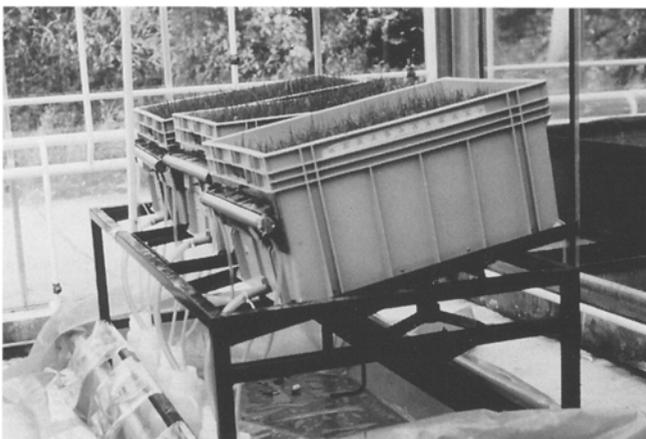
Fig. 1 Soil tilting table apparatus used to monitor the horizontal and vertical movement of *Cryptosporidium* in soil
