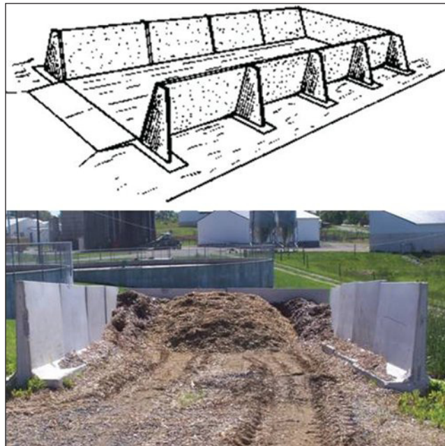
Figure 14. Bunker-type storage structure (Ogejo and Collins 2009).
